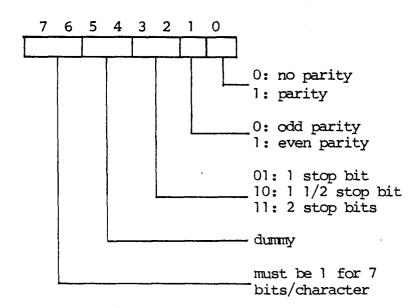
Recommended value for printers supplied by RC is 79 (2 stop bits, even parity).
