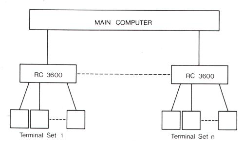
Various parts of this third kind of system might be utilized in a specific RC 3600 data collection system, and the connecting lines on the diagram above might represent data communications links or, simply, the manual transfer of, say, a paper tape from an accounting machine to a paper tape reader on an RC 3600. Editing and routing might be done at any or at all levels, and data conversion, editing, and routing could be done by the RC 3600's.
