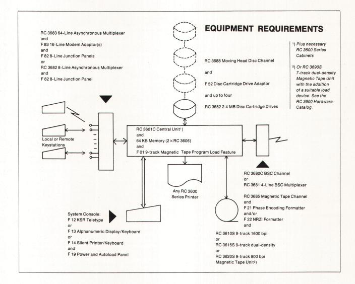
The RC 3600 data entry system enables the user to collect up to 9.3 million bytes of data on disc files from local and remote keystations under record format control. Completed data batches may be dumped to computer-compatible magnetic tape or transferred in RJE fashion to a central computer for processing. New record formats are easy to create, and any format included in the system can be accessed by all keystations simultaneously.
