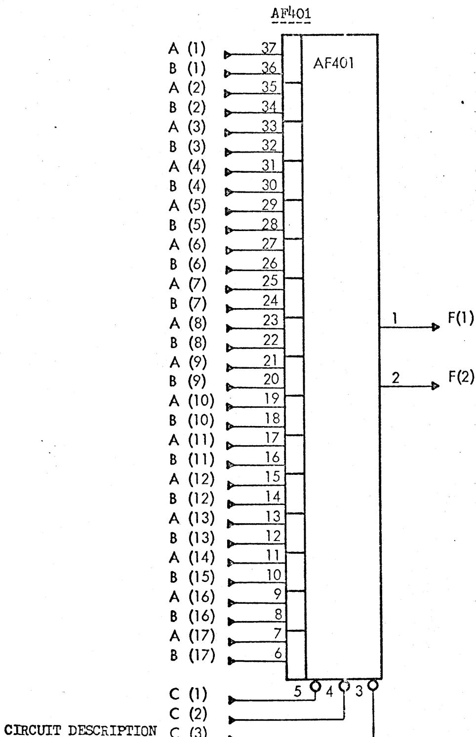
The AF<sup>4</sup>01 is an AND-OR element intended for digital multiplexer applications, e.g. bus systems. The element has 16x2 inputs, A(n), B(n), and 3 expander inputs, C(1), C(2), and C(3). The number of inputs may be increased by means of AND-NOR elements connected to the expander inputs. Output is available on 2 output terminals, F(1) and F(2).
