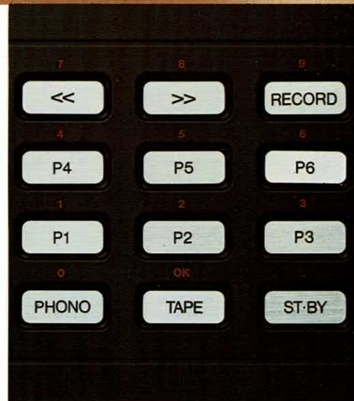
The central input unit comprises touch-sensitive buttons grouped together on a single panel to allow operation by one hand.
