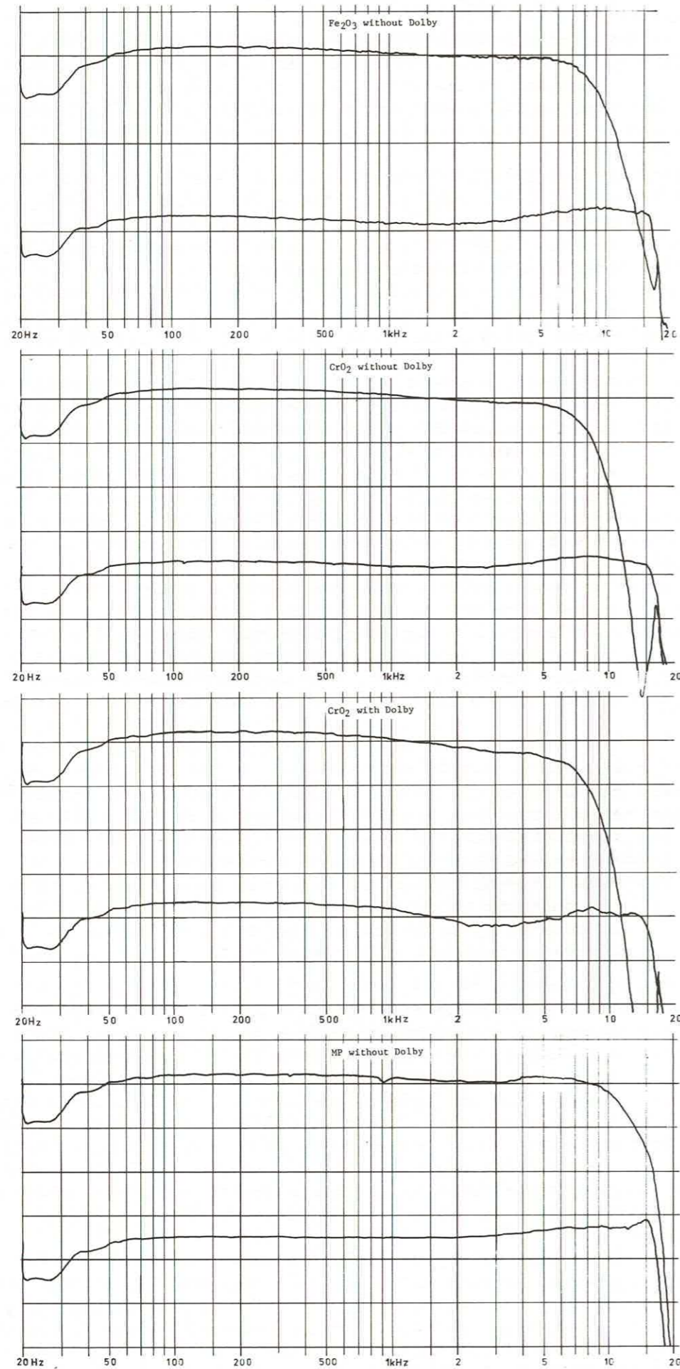
Fig. 8 - Record/Playback curves with oxide, crome and metal tape at Dolby level, and 20 dB below Dolby level. 5 db/division.
