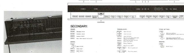
The Beomaster 5000 is the only component in the system having rear mounted sockets. The accompanying diagram shows facilities for PHONO, TAPE 1, TAPE 2, 240 Ohm Aerial, 75 Ohm Aerial, Main and extension loudspeakers, CD/AUX, two Relay sockets and RCA type sockets for PREAMP OUT. The PHONO, TAPE and AUX sockets are provided with both DIN type connectors and RCA connectors, the latter being used with products from other manufacturers.
