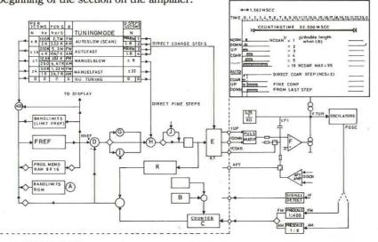
The block diagram is divided into two parts – on the left are the functions that are implimented in software in the microprocessor. On the right, are some of the basic hardware elements of the system.
