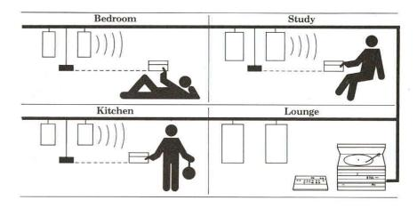
The main components of the system are located in the lounge – together with a Master Control Panel 5000. In the dining room, an additional pair of loud-speakers via Master Control Link are coupled to the main system.
