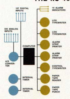
Regnecentralen is responsible for the hardware configuration and multiprogramming system at a new chemical plant, built by the Danish engineering company Haldor Topsøe at Pulawy in Poland. The plant, which is operated manually under continuous computer supervision, illustrates the application of the RC 4000 to industrial process control.
