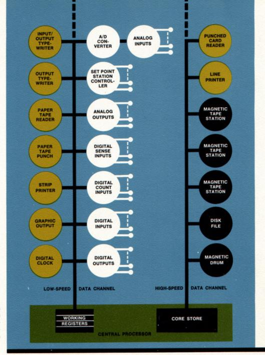
The block diagram illustrates a large-scale RC 4000 system configuration for process control, technical and scientific computation, and administrative data processing.
