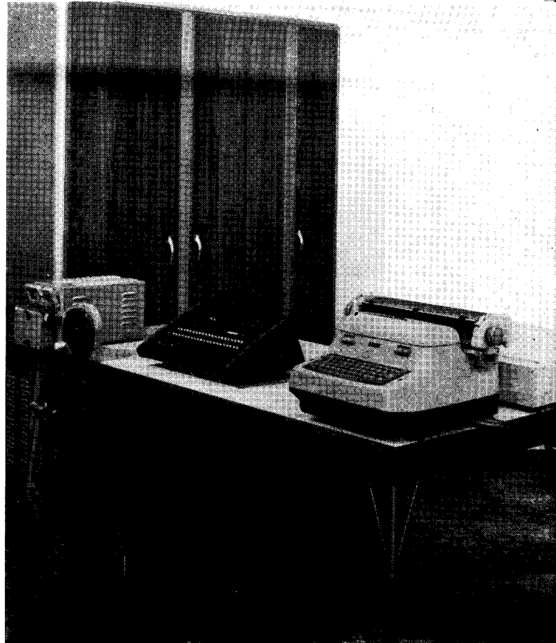
The central unit of GIER is accommodated in the cabinet in the background. On the table, to the left is a reader for paper tape, in the middle the control panel, to the right a typewriter for input and output, and behind the typewriter a rapid perforator for output.
