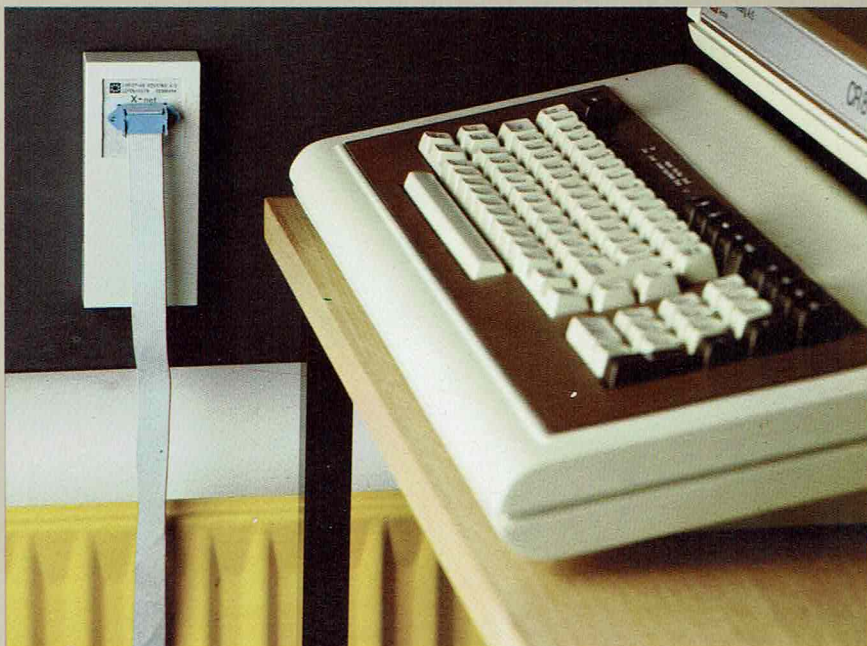
The CR8/PAM combination allows two-wire communication with PAM Data Acquisition and Control modules.
