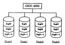
The major benefits of the striped disks are reduced access and seek time for higher performance of I/O operations in the system. However, due to the distribution of data onto 4 hard disks, the striped disk system causes a decrease in data safety. Because of this, a striped disk system is always implemented in combination with a mirrored disk system. Each of the 4 disks have their own mirror disk, and the 4 mirror disks also constitute a striped disk system.
