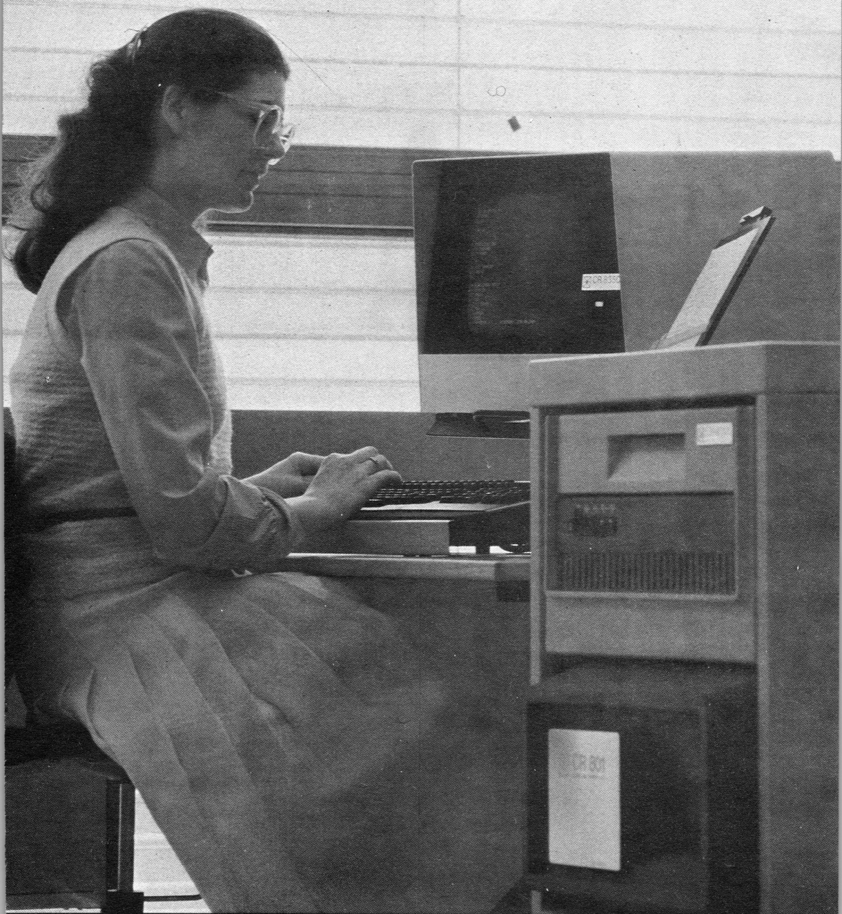
he CR80 MINI (Model 801) standard computer system for commercial EDP applications.
