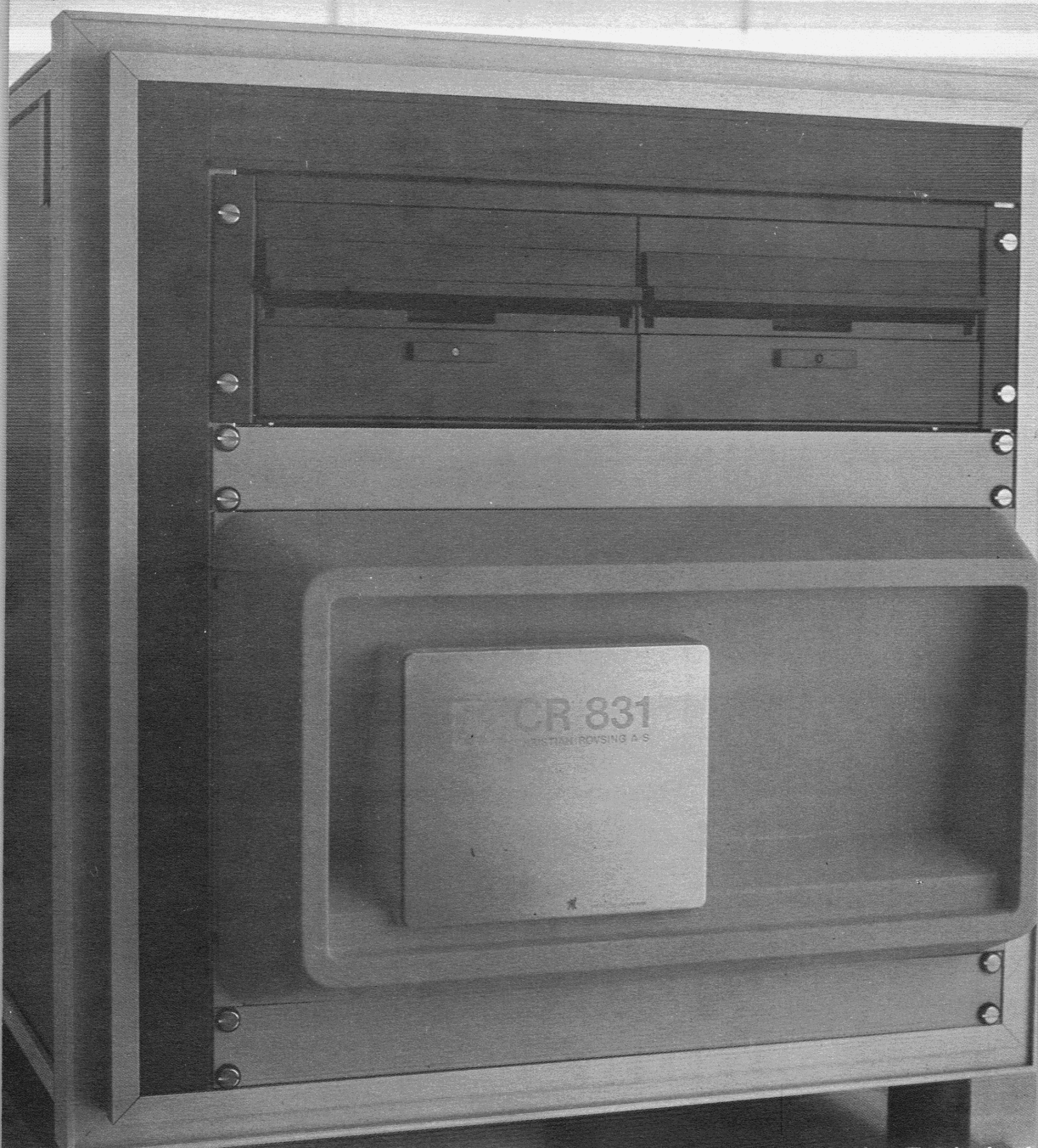
CR80 MINI (Model 831) Computer is particularly suited for medium size Technical or Communication applications. The snap-on front cover is easily removed during maintenance to give access to plug-in modules.
