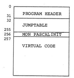
The execution of a CR80 PASCAL program starts with a monitor call which initializes the jumptable with the addresses of those subroutines in the runtime system which emulates the virtual instructions. The virtual code consists of JMPI S4 P8 instructions, possibly followed by parameters. Thus although the code is said to be virtual, it is basically CR80 machine code, and this fact makes insertion of "normal" CR80 machine code feasible.
