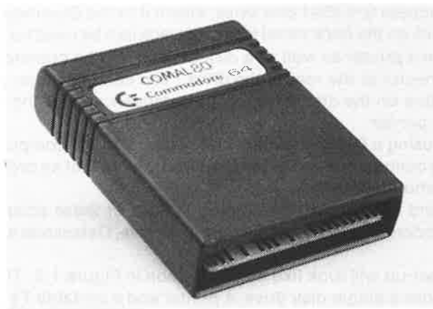
Figure 1.4: Your COMAL cartridge allows you to expand the power of your Commodore 64 without using additional memory. It fits into the cartridge slot at the rear of the Commodore 64 (or the top of an SX-64).
