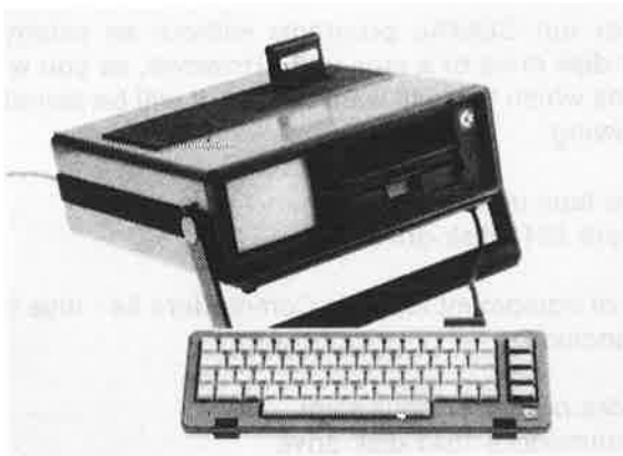
Figure 1.2: The Commodore SX-64 transportable computer is completely compatible with the Commodore 64. The SX-64 features a built-in color monitor and disk drive.
