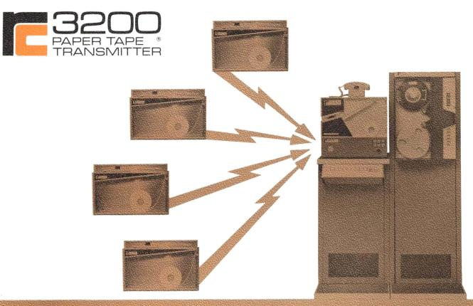
The RC 3200 permits transmission of paper tape data to an RC 3000 Converter System equipped with the RC 3100 Data Transmission Controller without restricting off-line conversion in conjunction with local data processing. A single RC 3000 can receive data from several RC 3200 transmitters, though not simultaneously.
