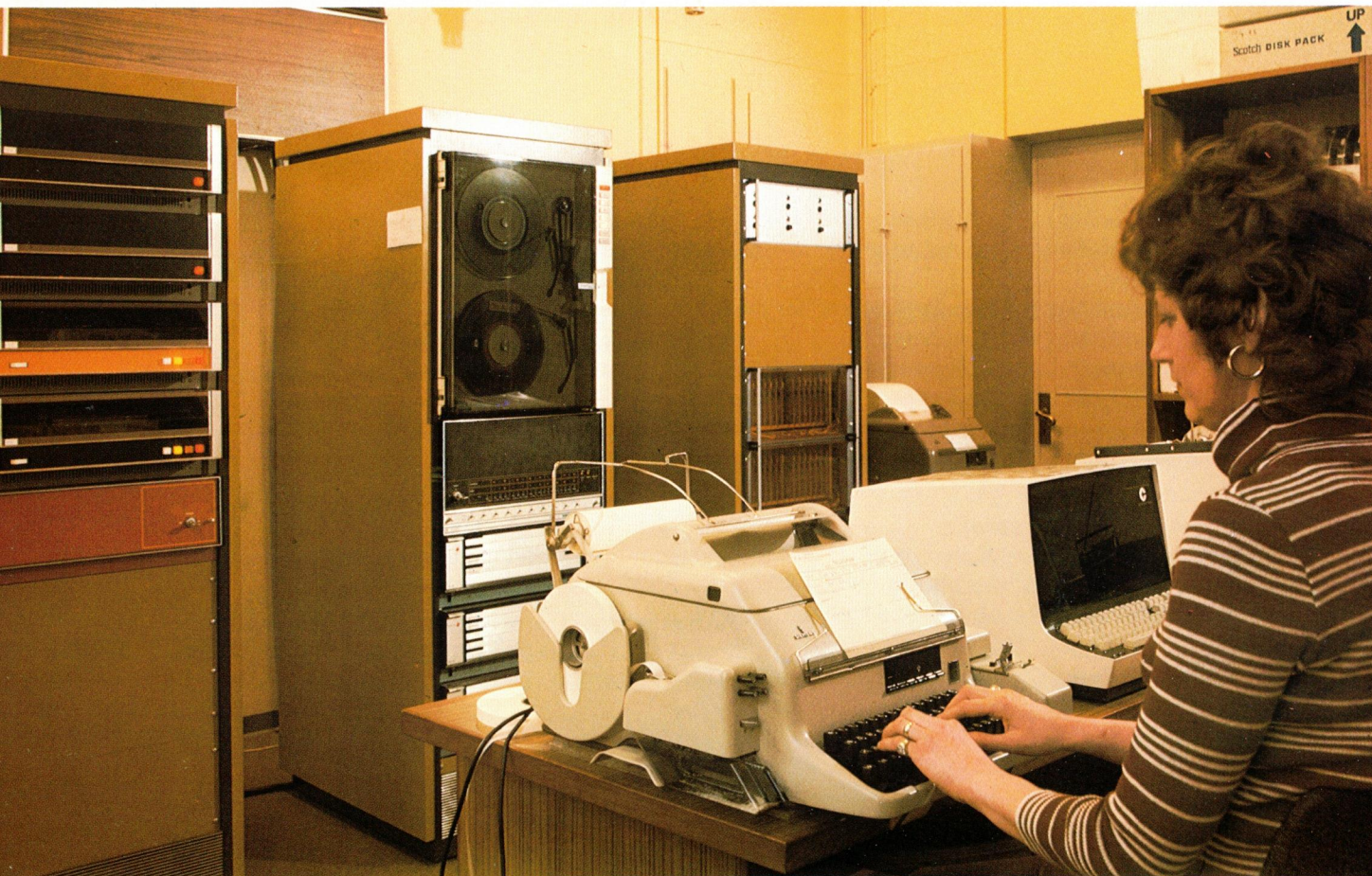
RC 7300 Message Switching System anvendes af ØK til styring af telextrafik. The RC 7300 Message Switching System is used by the East Asiatic Company to control telex traffic.
