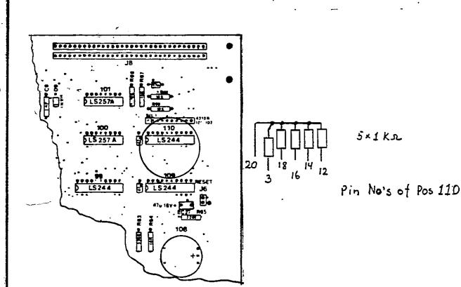
Max hight over board i 12 mm, which allows the use of Winchester adaptor.
