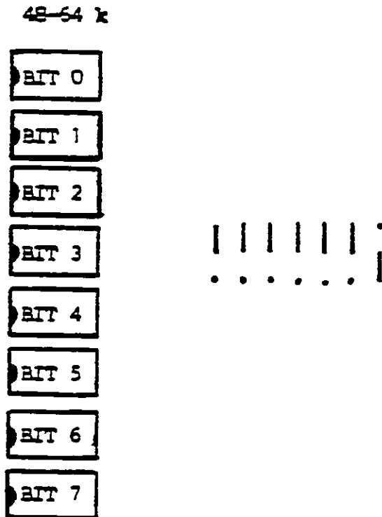
Figure 4: The switches 0-6 (here switch 6 is set).
