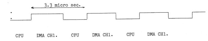
Timing for two DMA channels running:
