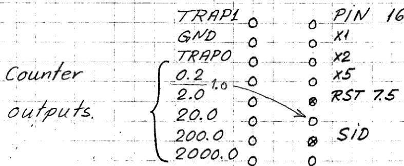
Times measured in ms \* Med 5MHz krystal
