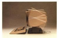
The display screen and keyboard of the RC 850 series are two separate units.
