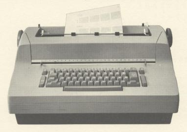
The input/output typewriter, which is equipped with a spherical typehead and pin-feed platen, has a maximum printing speed of 15 characters/second. The line width is 154 characters. The character set is a subset of the ISO 7-bit character set consisting of 88 graphics and 4 control characters.
