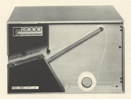
The paper tape reader has a reading speed of 2000 characters/second. It reads perforated tape of any opaque medium, accepting both. normal round-hole formats with 5, 7, and 8 tracks and the square-hole 6-track format. The tape is supplied from a free-running roll up to 300 m long, equivalent to approximately 120,000 characters. Data is transferred to the RC 4000 via the low-speed data channel. Parity checking can be performed in the paper tape reader controller.
