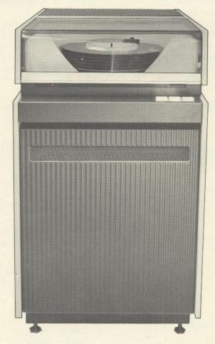
The magnetic disc store employs a removable disc pack with a capacity of 2,048,000 words of 24 bits. The disc pack, which is internationally compatible and can be replaced by other packs, has 10 recording surfaces and 200 cylinders (discrete positionings of the head cam).
