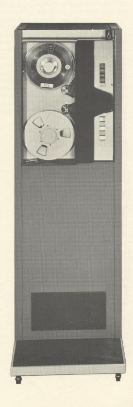
the high-speed data channel to or from the internal store of the RC 4000 by means of cycle stealing. The tape can be moved to upspace a file or block, backspace a file or block, or rewind or unload tape.
