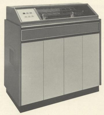
The line printer is a drum type device with 132 print positions. The print drum surface speed is approximately 1070 characters/second; with a 64-character drum this corresponds to a maximum printing speed of 1000 lines/minute.
