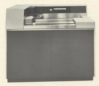
The punched card reader handles 12-row cards with 80 and 51 columns. Data can be transferred either via the low-speed data channel (column-by-column reading) by a sequence of standard input/output instructions, or via the high-speed data channel (card-by-card input) to the internal store.
