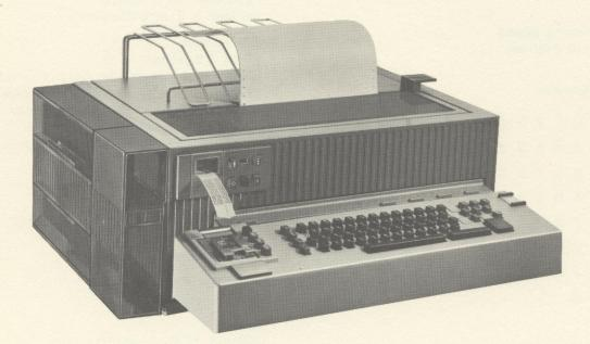
The teletypewriter terminal is an asynchronously operated printing and send/receive device providing a printing and transfer rate of 10 characters/second using the ISO/CCITT No. 5 (7-element) alphabet. The terminal includes a paper tape reader and punch, and, is connected to the low-speed data channel of the RC 4000 computer via the telemultiplexer, which can serve up to 24 simultaneously operating terminals.
