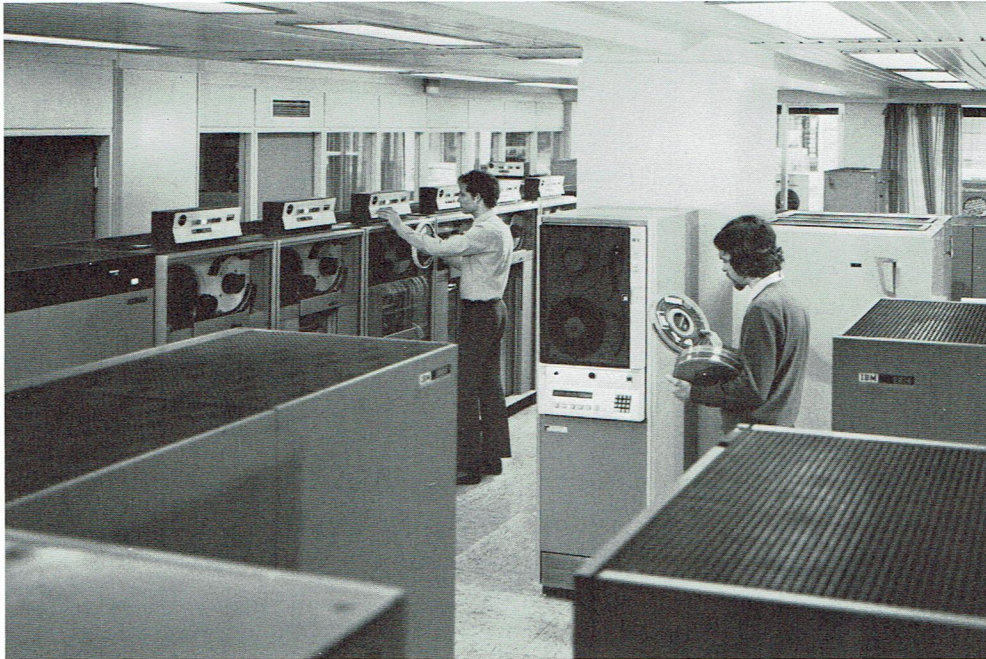
RC 3600 magnetic tape terminal at Sparekassernes Datacentraler, the data center of Denmark's largest savings bank network.
