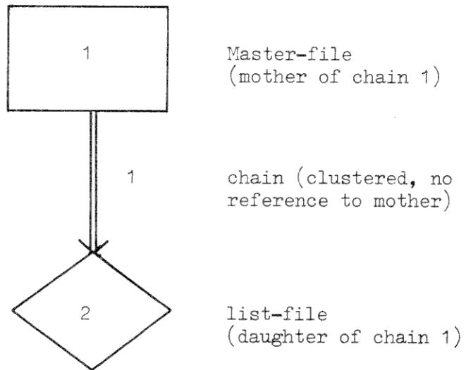
The diagram of fig. 1 shows a single master-file given the logical file-number 1, a single list-file given the logical file-number 2, and a single not headed chain, chain 1 of the configuration. The double arrow is used to indicate the chain, the daughter-records of which are clustered by the insert-1 procedure, exactly one double arrow must point to a list-file.
