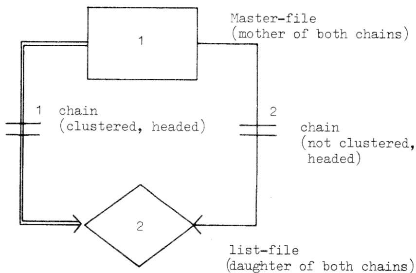
In fig. 2 the structure is extended by an extra chain-group, and both chain-groups are headed, i.e. each daughter-record holds a reference to the mother-record of the chain. This is specified by two bars crossing the arrows. Chain 1 is the clustered one.
