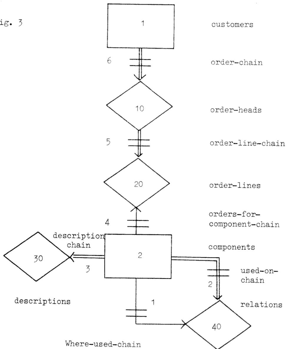
In fig. 3 an example is shown of the file-configuration of a sales-control system.
