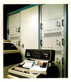
Utilizing the TDX bus all line multiplexing is done by interleaving of packets on the bus without loading of the CR80 minicomputer.
