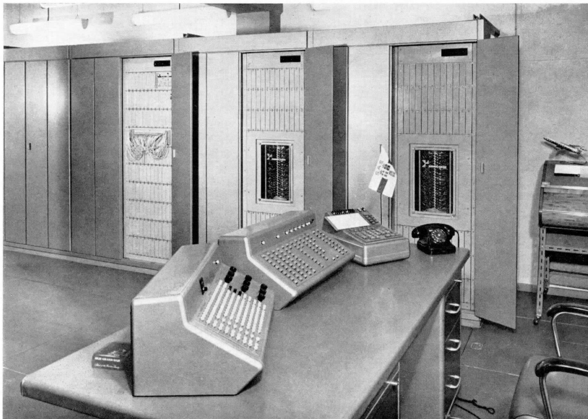
The seat availability computer was built by the Informatikwerk, a division of Standard Elektrik Lorenz A.G.
