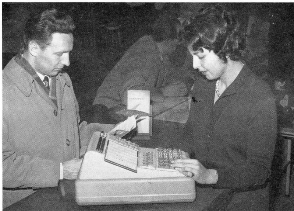
Inquiries concerning the availability of seats on any flight to be operated by S.A.S. during the next 70 days are entered on keysets located in the ticket sales offices
