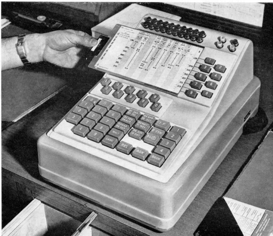
To make an inquiry, the operator first inserts an interrogation plate in the keyset and then depresses the appropriate data keys
