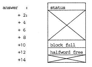
'block full' is the number of input blocks spooled for the pool, i.e. the number of blocks read by TEM, but not delivered to the user yet. 'halfword free' is the number of halfwords left for further input spooling.
