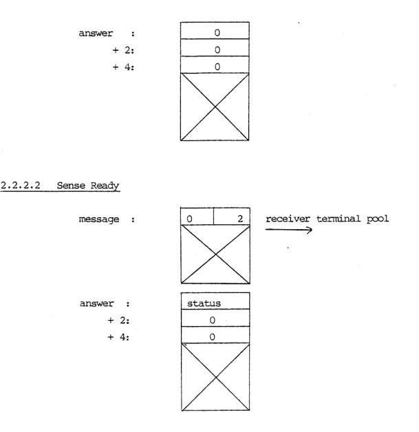
First input operations are initiated as described in 2.2.1.4. Then an answer from an external process is waited for. If data is ready the sense ready operation is answered with status = 0. Else the operation is returned with the answer delivered by the external process.
