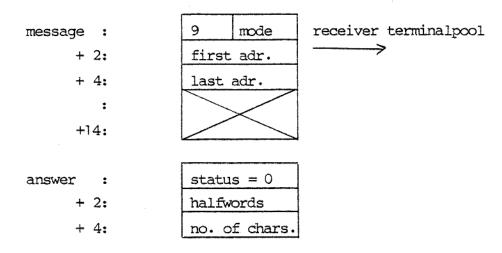
This operation is defined for links of type 0 only. The link addressed in the data area referenced by message (2:3) and message (4:5) is removed and created again. The data area specified will be handled by TEM in the same way as indata from the device. I.e. it will be delivered as data to the user process in a later input operation.
