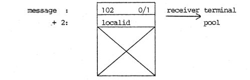
The operation removes a terminal link from a pool. The removal may be performed soft or hard, i.e. activities in progress may be terminated or suspended before the removal. In the first case message (1) must equal 0, in the second 1. The answer on a soft removal is given when the operation is initiated and tells thus nothing about the termination of the last activity on the link.
