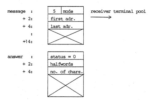
If the link exists, the result of the operation will be normal and status = 0. As the operation is taken over by TEM asynchronous with the working of the device, hard errors are not reported to the application.
