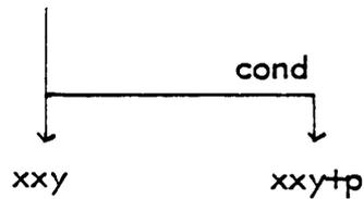
This is a partial (two) forks. The value of the condition directs the program flow towards right or left. Generally a true condition opens the branch on which it is written.
