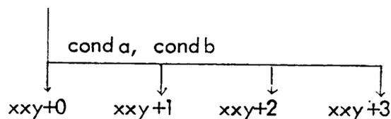
This is a full fork. Y has one of the values 0 or 4, and next instruction is found in address:  $xxy+2 + xxy+2 \times conda + condb$ , where conda and condb are the values of the selected conditions.
