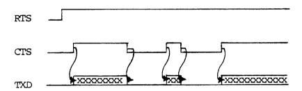
(Note: Following a cold boot, RTS ("ready to send") is switched on and sent by the RC855 to the receiving device. When the receiving device is ready, CTS ("clear to send") is switched on and sent to the RC855. The RC855 can transmit as long as CTS is on. Transmission takes place on line TXD.)
