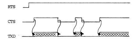
(Note: Whenever the RC855 attempts transmission via the printer port, RTS ("ready to send") is switched on and sent to the printer. When the printer is ready to start receiving, CTS ("clear to send") is switched on and sent to the RC855. The RC855 can transmit as long as CTS is on. Transmission takes place on line TXD.)
