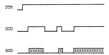
(Note: Whenever a cold boot takes place, DTR ("data terminal ready") is switched on and sent by the RC855 to the transmitting device. The RC855 receiver is not enabled, however, until DCD ("data carrier detect") has been sent to the RC855 by the transmitting device. RXD is the line on which the RC855 will receive data from the transmitting device.)
