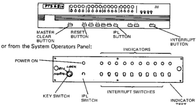
Note: the illustration above is an example of one type of Full Panel; exact layout may differ slightly between models.
