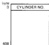
A cylinder number is written in the first word of every sector when the disk is initially formatted by the utility PM6800. It contains the number of the cylinder in which the sector is located. It is used by the Monitor to check if a seek operation has been successful or not.
