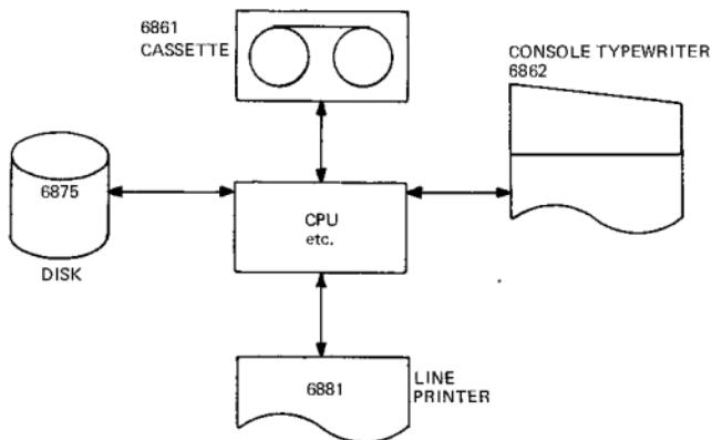
Note: It is possible to replace the cassette unit with a flexible disk drive, if required.
