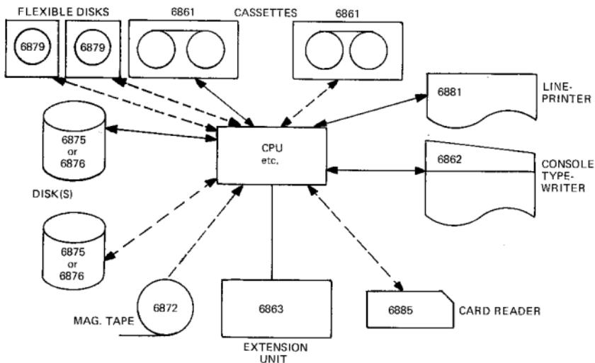
Note: The 6875 and 6876 disk units may be used in a mixed configuration, to a maximum of two drives in total.
