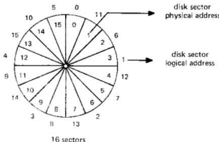
Physical addresses are used by the Monitor when reporting disk errors on the console typewriter. In all other cases the logical address is used. For example, all data management functions refer to logical addresses and when a disk dump is made the sectors are printed in their logical sequence.
