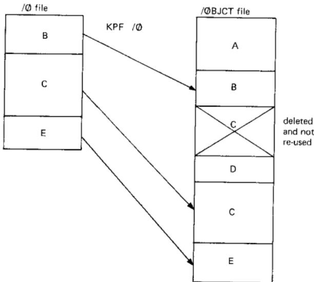
In the above example the new module B is the same size as the old module B and is thus written over the old module. The new module C is larger than the old module C so the old module is deleted and the new module is written after the last module in the file. The new module E did not exist in the /ØBJCT file prior to the KPF. It is therefore added at the end of the file.
