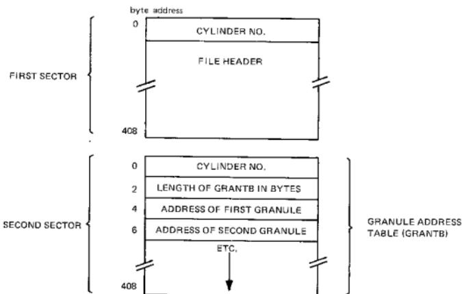
A GRANTB is set up each time a disk file is assigned. As the file is created the address of each granule used by the file is entered in the table. The last address in GRANTB is followed by a word containing /0000.
