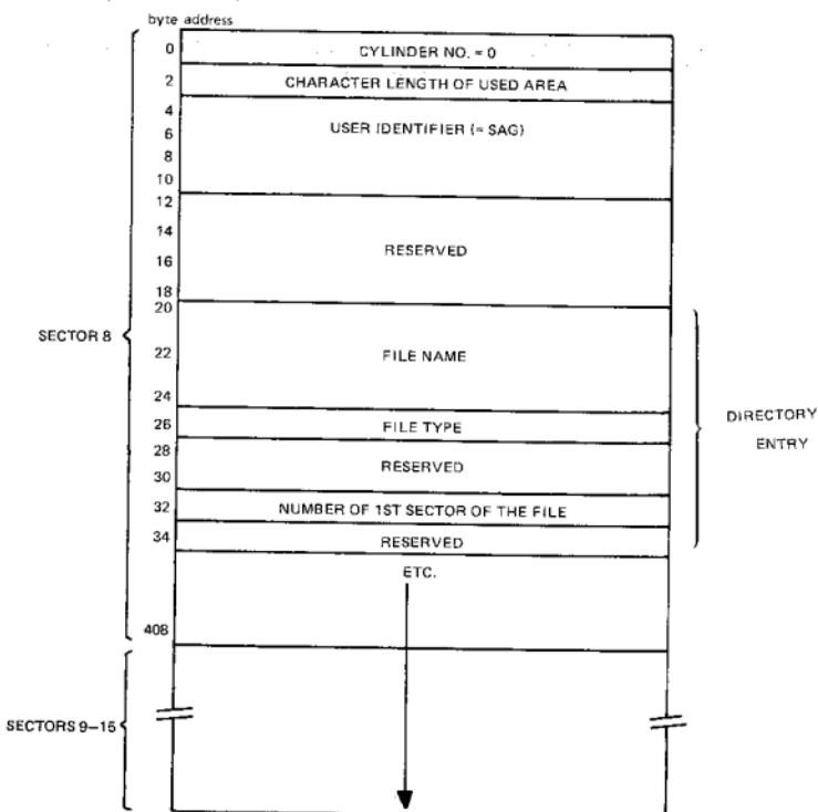
There is one eight word entry in the directory for each file in the library of userid SAG. Each entry contains the file name, the file type and the number of the first sector of the file. The format of the entry is shown in the above diagram (bytes 20 to 35).
