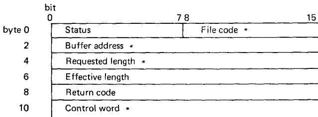
The ECB must be reserved in the application program via the DATA and/or RES directives. The fields marked with an asterisk in the above diagram must be set by the user although the control word can be set by the driver on return e.g. order code /00, Test Status returns the current status of the device to the control word. The remaining fields are set by the drivers.
