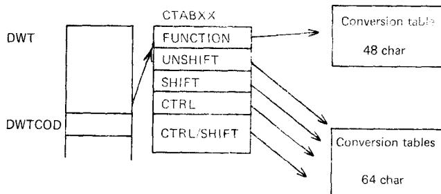
Each entry not zero in CTABXX gives the address to the code conversion table. The conversion tables may be used common for several keyboards. One or more conversion tables may be excluded by setting zero or UNSHIFT in corresponding entry in table CTABXX. Zero means no conversion and UNSHIFT conversion according to the UNSHIFT-table.
