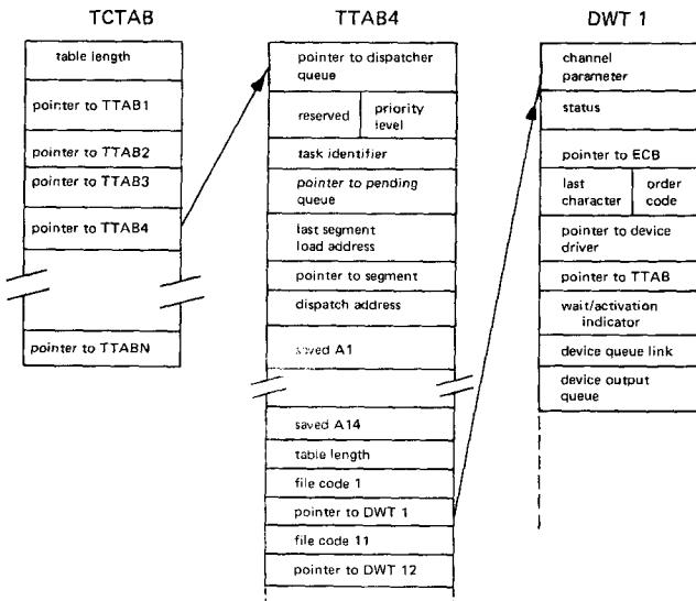
There is one TCTAB in the system. It points to each TTAB in the system. There is one TTAB per task. TTAB points to each DWT used by the task. There is one DWT for each device in the system, though the CREDIT debugger requires a second DWT for the SOP switches.
