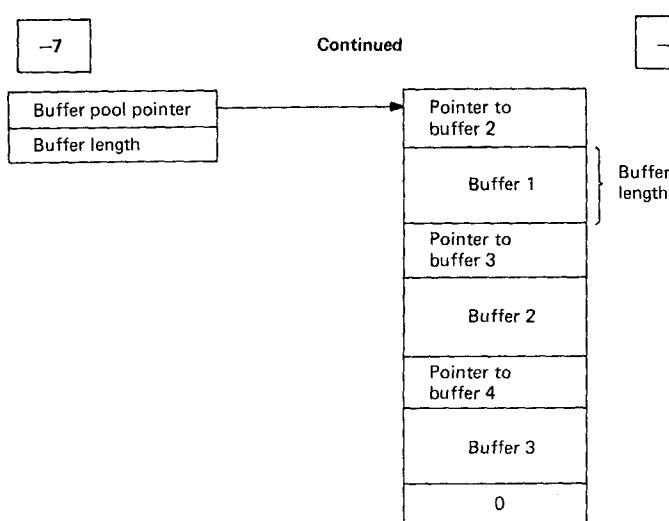
The pointers at the start of each buffer must be set up by the application program before the first GET BUFFER request. However, they need not be maintained by application tasks. That is, when a GET BUFFER request is made an area of memory, including the pointer, is allocated to the task. The task may overwrite the buffer pointer in addition to the associated buffer. When a release buffer request is made the pointers are automatically regenerated by the Monitor.
