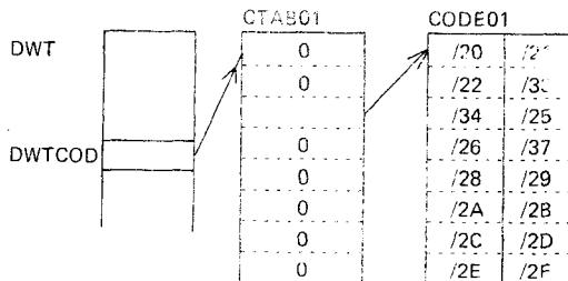
DWTCOD of the device work table holds an address of an 8-word table CTAB01, indicating the columns to be converted. (DWTCOD) = 0 means no conversion for this keyboard.
