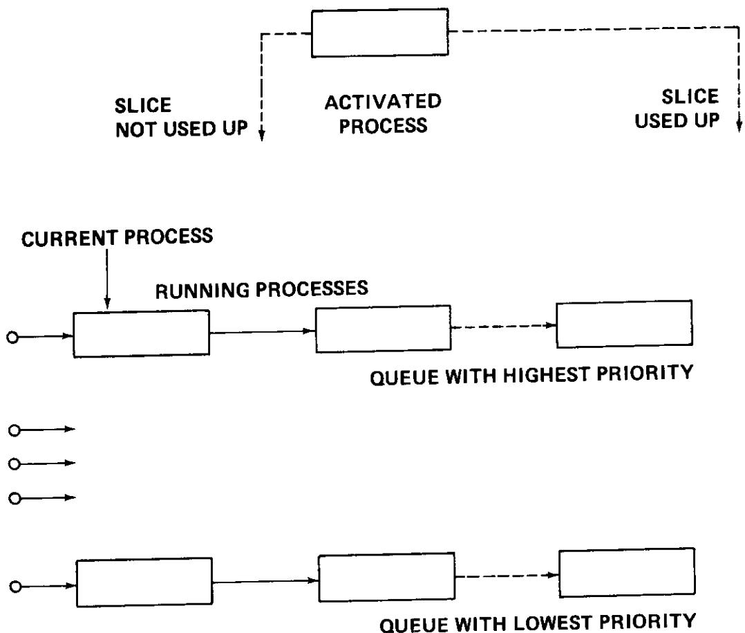
Over and beyond the round-robin scheduling of the monitor, one can assign priorities to internal processes. Each priority level has its own time-slice queue, in which processes run on a round-robin basis. When the queue with the highest priority is empty, i.e. when all of the processes are either waiting or stopped, process execution continues in the queue on the next highest level.
