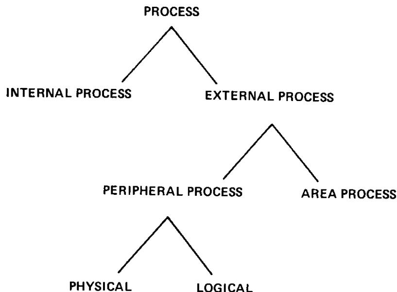
As may be seen from the figure above, a fundamental distinction is made between internal processes and external processes; the former correspond roughly to program execution, the latter to input/output.
