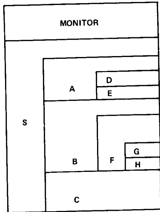
This family tree of processes can be extended to any level, subject only to a limitation on the total number of processes. At present the maximum number of internal processes which can be created under the basic operating system is 21.
