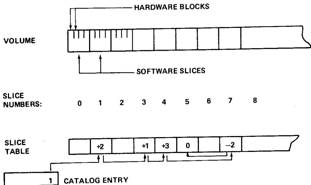
The number of the first slice is defined in the catalog entry describing the file. Free slices have a unique value in the slice table. When a file is extended, a free slice-table halfword is linked to the end of the chain representing the file. Once a volume is mounted, its slice table is kept in the primary store for fast reference. Whenever a permanent file is extended or reduced, the slice table is copied to the volume as a safety measure.
