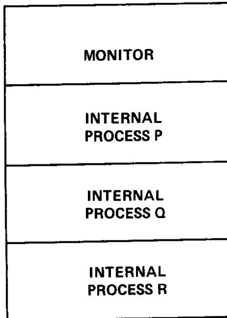
Later, in Chapter 6, we shall explain how internal processes are created and how programs are loaded into them. Here it is sufficient to point out that an internal process occupies a contiguous storage area of a fixed size during its entire lifetime.
