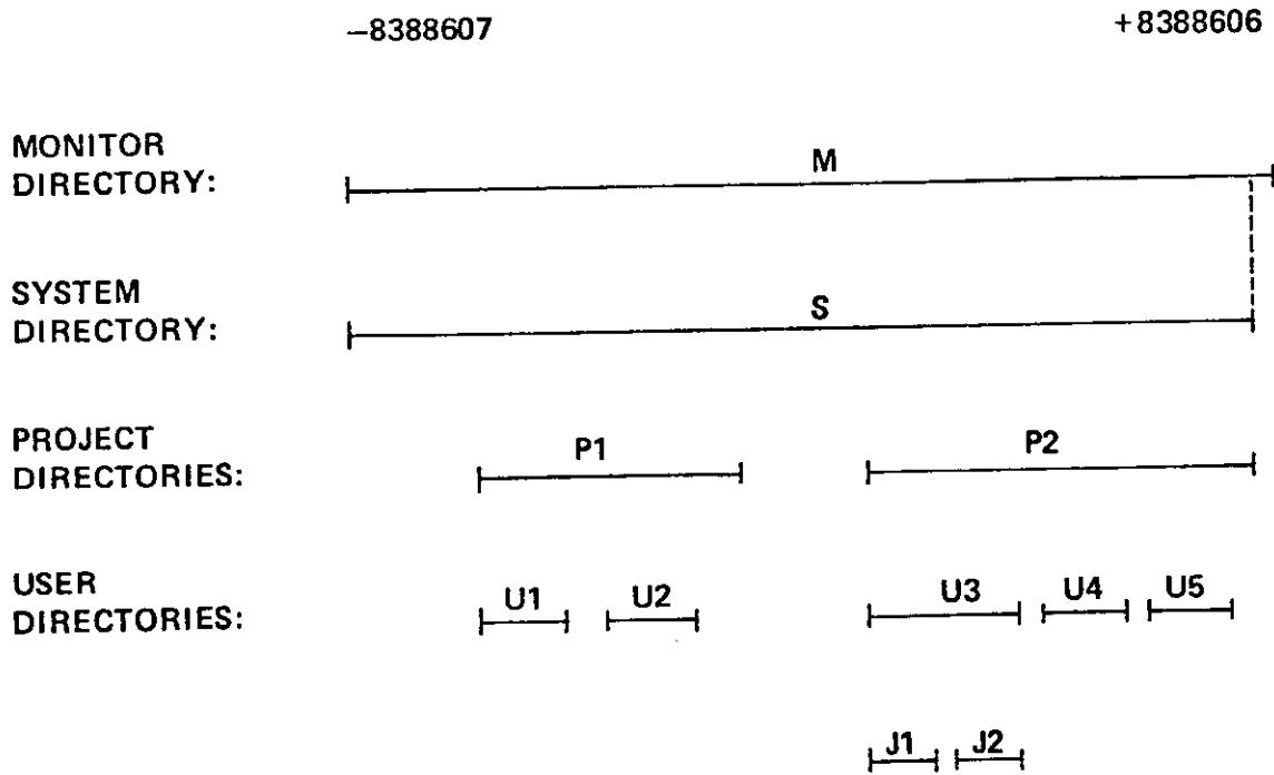
It has already been stated that a "directory" is simply a set of files with a given name base. Within the monitor these sets of files are implemented by means of the various bases that are associated with files and internal processes. Thus a "project directory" from the viewpoint of a process is expressed by its max base and a "user directory" by its current catalog base.
