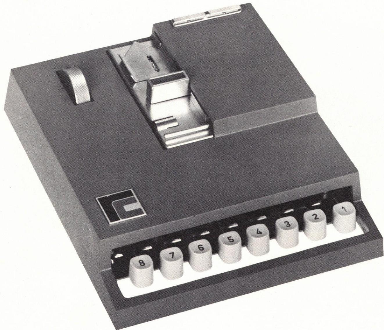
The RC Mechanical Punch provides accurate and convenient punching of 5 and 8 track paper tapes. The keys of the punch correspond to tape tracks, beginning with the least significant bit at the right. As each track can be punched individually, it is possible to create any existing code.
