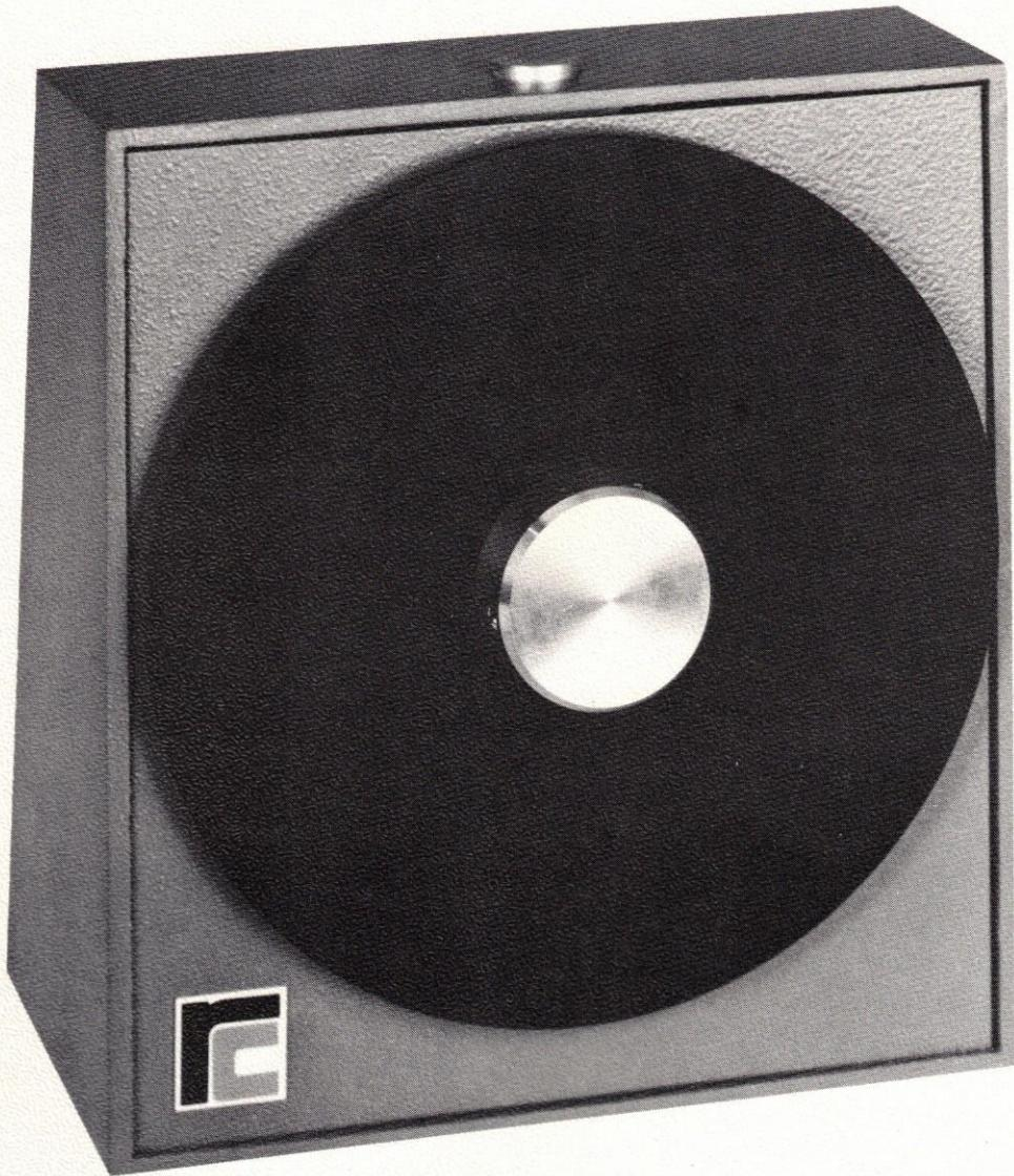
The RC Electric Tape Winder provides high-speed winding of 5, 6, 7, and 8 track paper tapes on cardboard cores. Its specially constructed motor has maximum torque when started, and its winding speed can be varied from 0 to 2400 revolutions/minute by manual braking.
