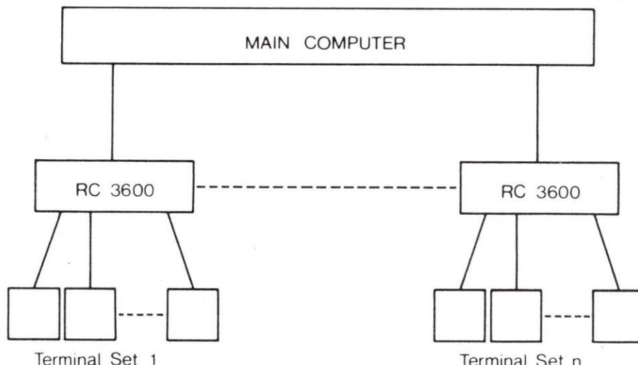
Various parts of this third kind of system might be utilized in a specific RC 3600 data collection system, and the connecting lines on the diagram above might represent data communications links or, simply, the manual transfer of, say, a paper tape from an accounting machine to a paper tape reader on an RC 3600. Editing and routing might be done at any or at all levels, and data conversion, editing, and routing could be done by the RC 3600's.
