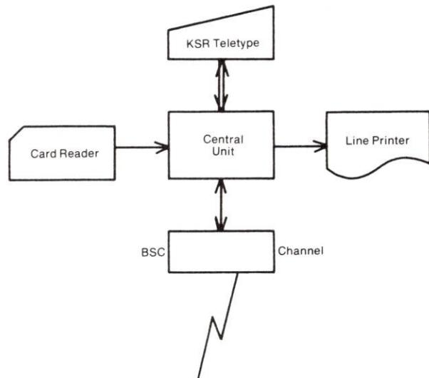
Data Communications Configuration (Point-to-Point Communications System)
