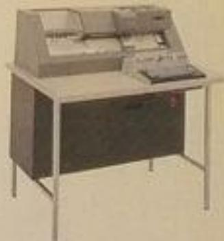
The 3248 Card Data Reader makes the 36-column tape used with System/3 Model 10.
